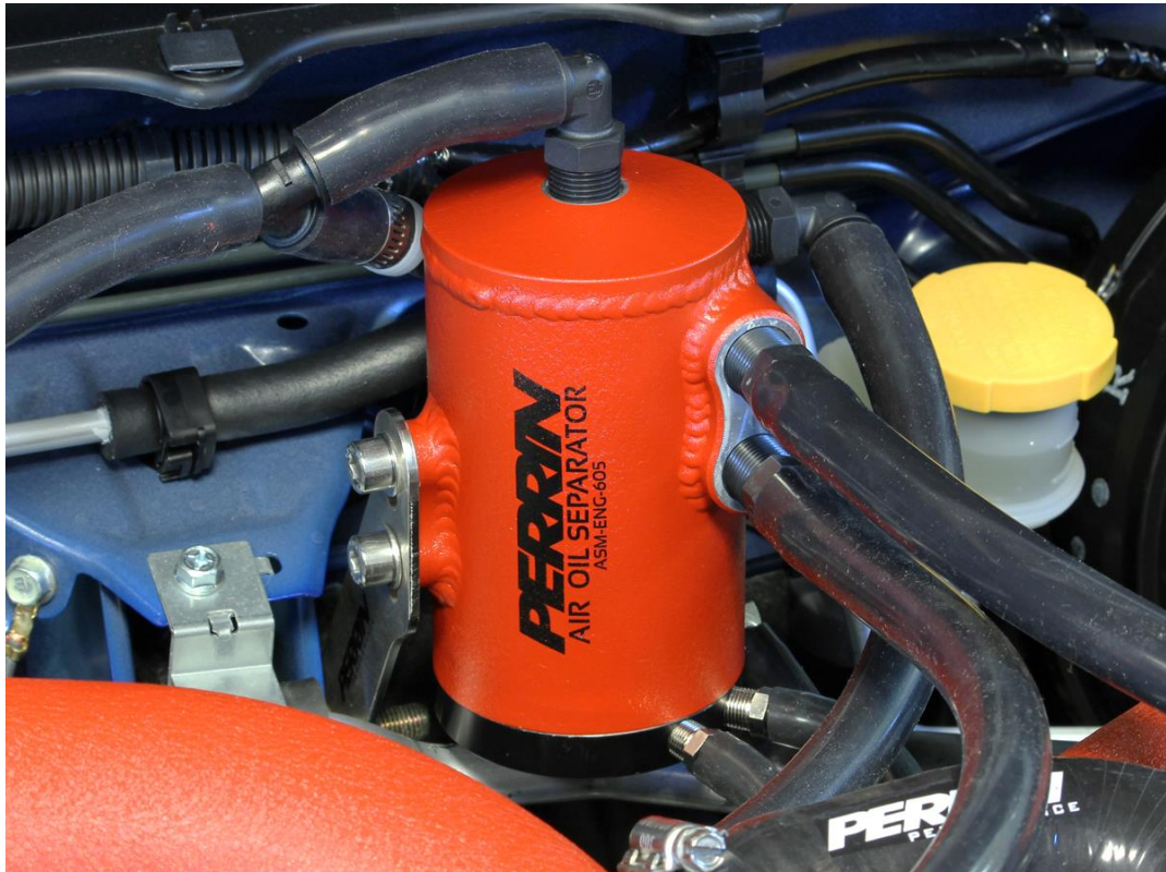
Above shows completed installation of AOS on a car with a PERRIN FMIC installed.
