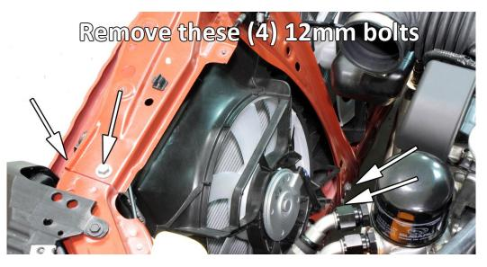
8. Lift up on left side of radiator support (leaving intake air diverter in place) and place PERRIN intake tube under support as shown below. Make sure that tab on PERRIN intake is in front of radiator support and closely lines up to threaded M6 hole shown below. Carefully set radiator support back down and reinstall (4) 12mm bolts removed earlier.
