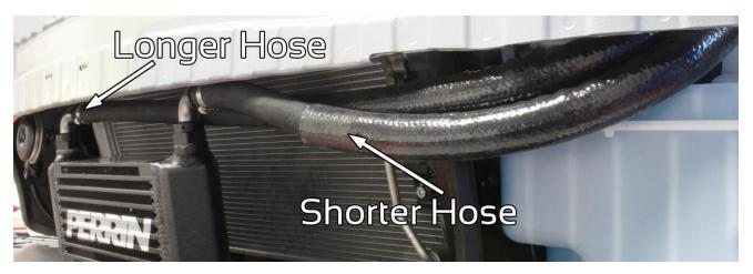
25. Run supplied oil lines through hole in chassis as shown below making sure to leave 45 degree bent fittings toward thermostat housing. Make sure and route hoses the same way as shown in pictures. This is done to provide the smoothest path from the oil cooler to the thermostat housing.
