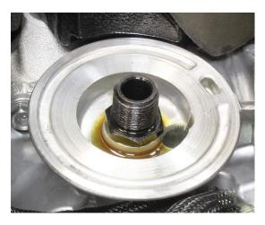
27. Install thermostat housing adapter over the male-to-male adapter so that both open ports are facing the front of the car. NOTE: Make sure to place rubber seal down toward the engine.
