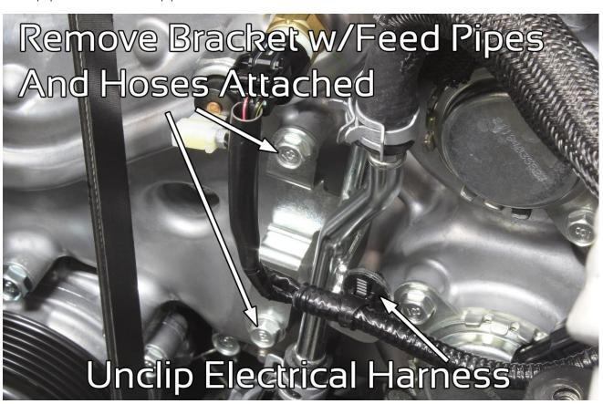
9. Locate and remove (2) M6 bolts securing steel bracket with the coolant pipes on front of engine. Unclip wire harness from bracket.
