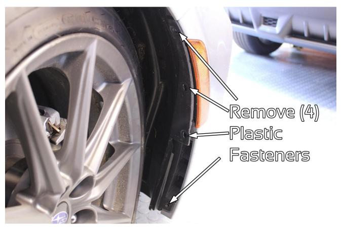
c. Under car, locate and remove and (8) plastic fasteners holding lower portion of bumper skin to car.
