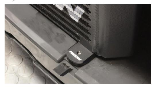
23. Install M6 fender washer then M8 fender washer onto supplied M6 bolts. Pull down lower splash guard and install them up through the holes in the splash guard and into the PERRIN Oil Cooler Brackets. Tighten bolts to roughly 10-15ft-lbs of torque.
