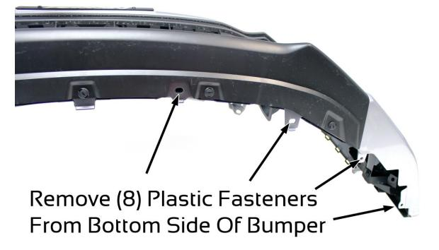
d. Starting at corners next to side marker lights, pull bumper straight and away from car to unsnap from chassis. Do this to one side then the other before proceeding to next step.
