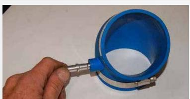
Install the provided 3/8" diameter by 2" long aluminum adapter tube. Push the long end into the port on the side of the provided blue hose connector. This is the new breather tube connection point.
