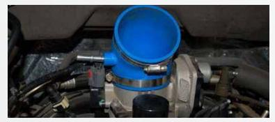
Install the blue connector and two clamps onto the throttle body.
