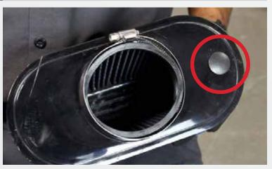
Install the sponge trimming onto the BBK Cold Air Intake shield and install the supplied plug into the BBK Air Filter.
