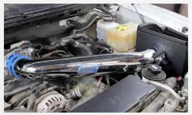
Install the blue BBK Coupler and BBK Intake Tube to the throttle body.
