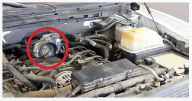
Unclip the three clips at the air box and remove the entire system out of the vehicle.
