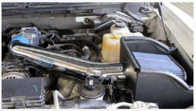
Install the supplied Air Filter, plug in the MAF Sensor and be sure all the clamps are tight.
