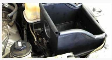
Place the cold air shield into the vehicle on the bottom half of the factory air box and use the three original clamps to secure the shield.
