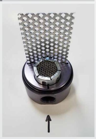
Make sure when running hose to plastic fitting on intake side you connect the hose to the filtered side of oil separator kit this is the draw side. It helps with filtering any debris thru oil.
