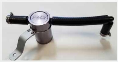
Using supplied components assemble oil separator kit as shown in pic. Using the two supplied clamps at engine connections only.
