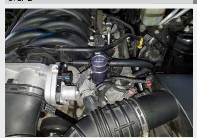
Now on the driver side engine compartment remove factory PCV hose and install BBK oil separator kit and mounting the bracket to factory 6mm bolton intake manifold behind factory throttle body as shown in picture. Using supplied two clamps for hose connections at intake and valve cover.
