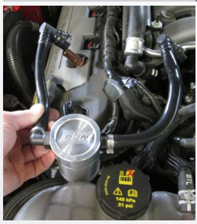
Install the (2) vacuum hoses supplied in the kit onto the BBK oil separator canister.
