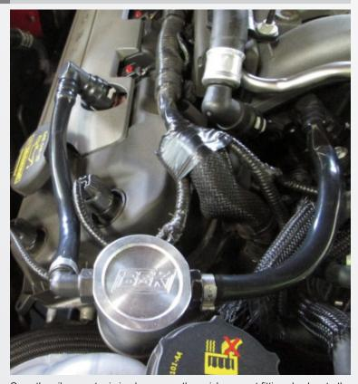
Once the oil separator is in place press the quick connect fittings back onto the barb fitting on the intake and valve cover.
