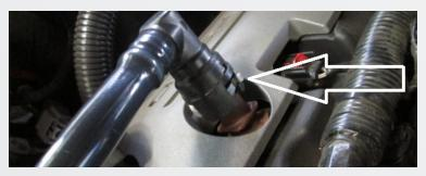
Release the (2) quick connect fitting on the intake manifold and valve cover and remove the vacuum hose from the vehicle.
