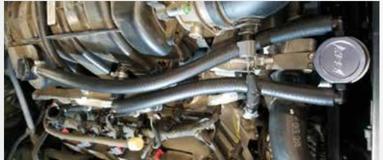
Assemble Oil Separator Kit as shown in pic making sure hose that runs to the intake manifold is the draw side shown in pic. Then remove factory engine cover and factory PCV hose. Now mount Oil Separator Kit using existing engine stud and hoses with supplied nut and clamps as shown in pic.
