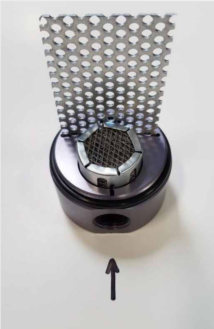
From this side of the oil separator the hose will go to intake.
