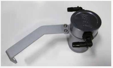
Assemble oil separator by installing o-ring bracket onto separator by removing cap. Now screw cap back down aiming towards top of BBK logo also install supplied fittings using 17mm wrench in the same direction. Now install bracket and Allen bolts using a 3/32 Allen wrench as show in photo.
