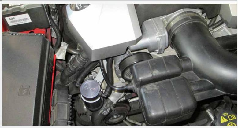
Now double check all connections then install throttle body, air box and engine cover.
