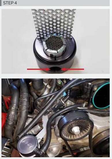
Now install new BBK oil separator assembly as shown in picture and tighten nut. When running hoses to oil separator run your first hose from the plastic fitting on intake manifold to the filtered side of oil separator as shown in picture. Then run the other hose from steel tube below intake manifold to the other side of the oil separator. This is the pressure side.
