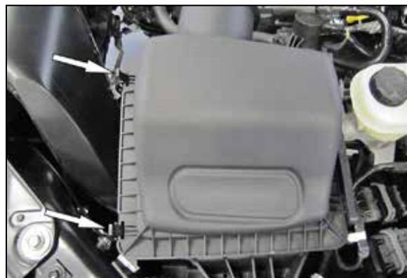
4. Unclip the upper air filter housing clips and remove the upper air filter housing and factory air filter.
