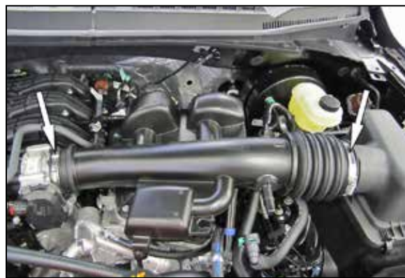
3. Loosen the hose clamps that secure the intake tube, unclip the coolant line and vent hose clip and then remove the factory intake tube. NOTE: K&N Engineering, Inc., recommends that customers do not discard factory air intake.
