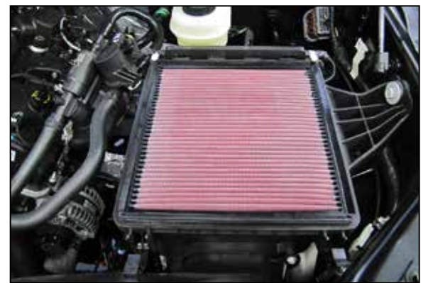
5. Install the K&N® air filter and then reinstall the air filter housing do not secure the lid at this time.
