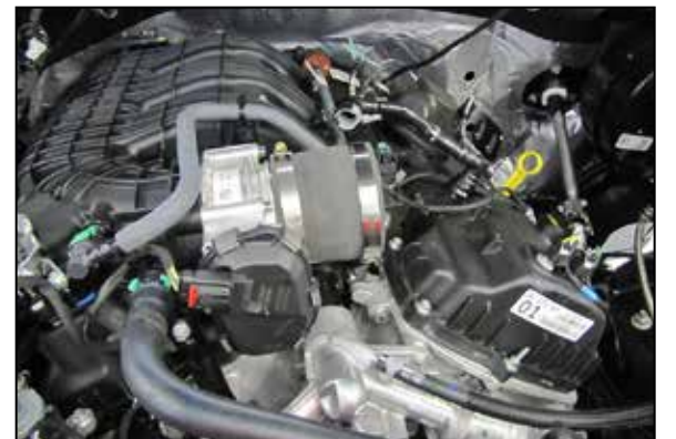
6. Install the provided coupling hose (084055) onto the throttle body and secure with the provided hose clamp.
