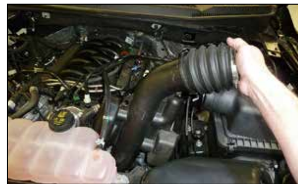
5. Remove the factory intake tube from the vehicle.
