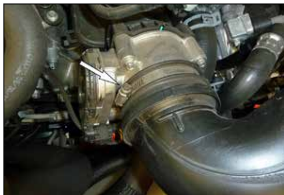
3. Loosen the hose clamp that secures the intake tube to the throttle body.
