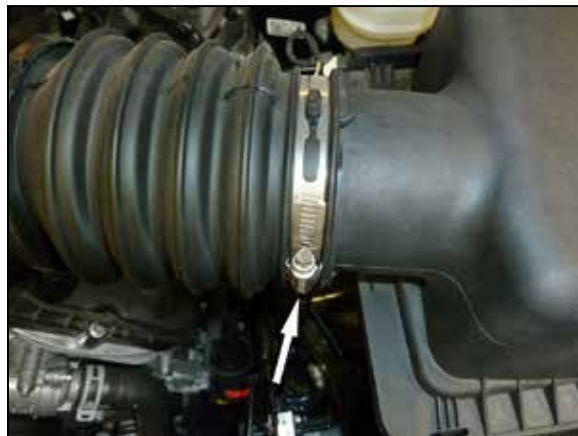
4. Loosen the hose clamp that secures the intake tube to the air filter housing.
