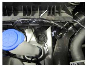
4.Remove the front air filter housing mounting bolt and unhook the wiring harness from the housing.
