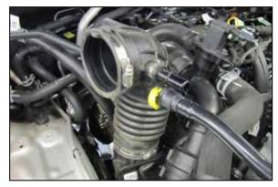
7. Loosen the hose clamp that secures the intake hose to the plenum and then remove the hose from the vehicle.
