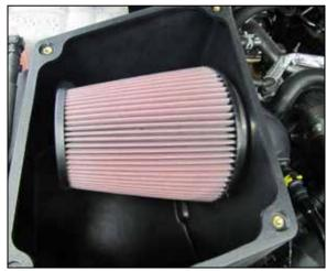
15. Install the K&N air filter onto the filter adapter
