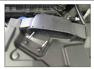
3. Remove the two bolts that secure the factory fresh air intake duct and then remove the duct from the vehicle.
