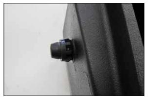
12. Remove the factory air filter housing mounting post and install it onto the K&N air filter housing as
