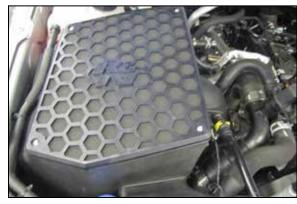
16. Install the filter lid assembly onto the air filter housing and secure with the provided hardware.
