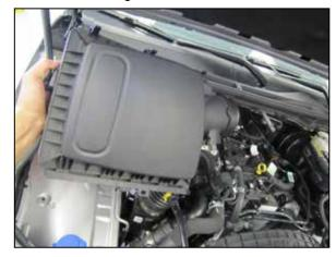
6. Remove the air filter housing from the vehicle. NOTE: K&N Engineering, Inc., recommends that customers do not discard factory air intake.
