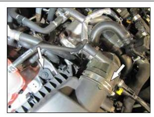
5. Remove the rear air filter housing mounting bolt and loosen the hose clamp that secures the intake hose to the housing.
