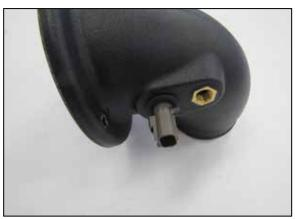
9. Remove the inlet air temperature sensor from the factory housing. Remove the O-Ring from the sensor and then install the sensor into the K&N intake tube using the provided grommet.
