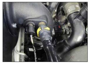
14. Reconnect the inlet air temperature sensor electrical connection and connect the crank case vent line to the fitting installed into the K&N intake tube.
