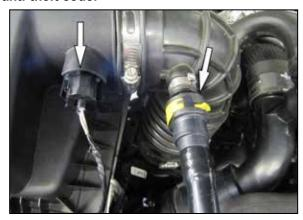
2. Disconnect the inlet air temperature sensor electrical connection and disconnect the crank case vent line from the factory intake tube.
