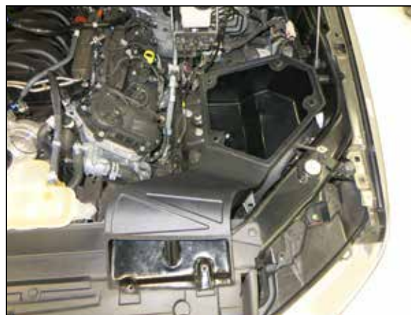
12. Install the K&N lower air filter housing assembly into the vehicle.
