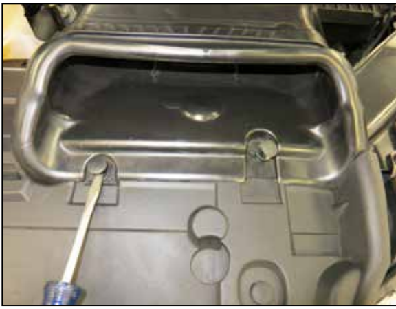
5. Pry up the push-pin locks that secure the fresh air intake duct and remove the pins.
