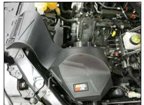
18. Install the upper housing assembly onto the lower housing so the mounting posts insert into the grommets.
