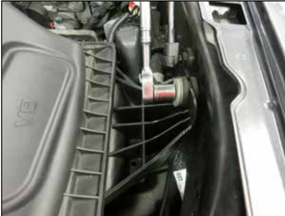
6. Remove the bolt that secures the factory air filter housing to the inner fender.
