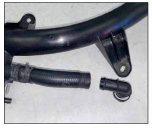
21. Release the spring clamp that secures the quick connect fitting onto the BOV hose and then remove the fitting from the hose.
