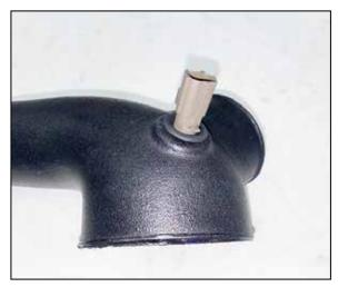
17. Remove the IAT sensor from the factory intake tube and then install it into the K&N intake tube using the provided grommet. **NOTE: The IAT** sensor is fragile, use care while handling the sensor so as not to damage it.
