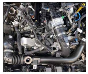
5. Loosen the hose clamps that secure the driver's side intake tube.
