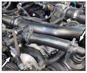
3. Release the BOV hose quick connect fitting and disconnect the BOV hose from the intake tube. Then disconnect BOV electrical connection and unhook the wiring harness from the mounting post.
