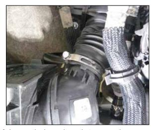
9. Loosen the hose clamp that secures the passenger side intake hose to the air filter housing and then remove the factory air filter housing from the vehicle.
