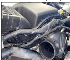
8. Unhook the wiring harness and coolant hoses from the air filter housing.
