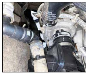
10. Remove the bolt on the bottom side of the passenger side intake tube that secures the tube to the engine. Then release the spring clamp that secures the intake tube to the turbo and remove the passenger side intake tube. **NOTE: The spring clamp is difficult to release with the tabs positioned towards the bottom of the turbo inlet.**
