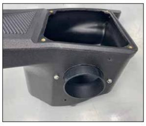
13. Install the provided filter adapter into the K&N air filter housing and secure with the provided hardware.
