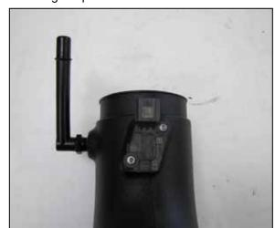
27. Install the CCV fitting into the K&N intake tube as shown.
