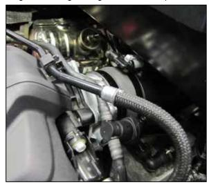
31. Reconnect the mass air sensor electrical connection.
