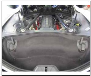
32. Reinstall the filter access panel, carpet and top stowage mounts using the factory hardware.
