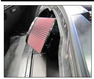
29. Push the intake tube towards the rear of the vehicle, install the filter onto the tube and secure with the provided hose clamp. Be sure to check the alignment before tightening the hose clamp, when the intake tube is installed the filter should sit horizontal.
