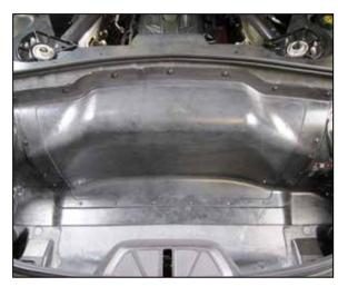
4. Remove the nineteen bolts that secure the air filter access panel and then remove the panel and set aside.
