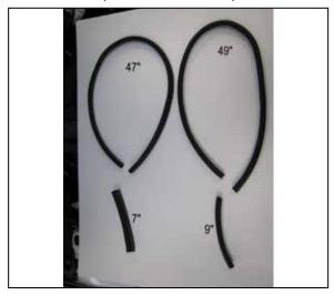
19. Cut the two provided edge trim into sections as shown.
