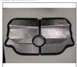
21. Peel the backing off the heat barrier and then apply the barrier to the engine side of the heat shield as shown. After the heat barrier is installed, use a knife or similar tool to cut out all of the mounting holes in the heat shield through the heat barrier.
