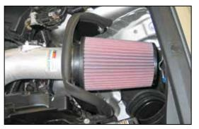
25. Install the K&N $^{\mbox{\scriptsize \$}}$  filter and secure with provided hose clamp.
