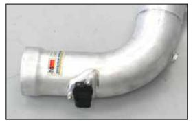
21. Install the mass air sensor into the intake tube and secure with the provided hardware.
