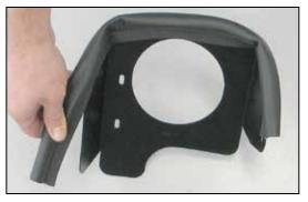
16. Install the provided edge trim onto the heat shield as shown.
