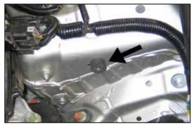
17. Install the provided rubber mounted stud into the air box mounting bracket location as shown.
