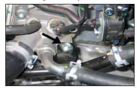
13. Remove the bolt shown that secures the heater hose pipe to the thermostat housing.
