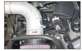
14. Secure bracket number 083121 to the thermostats housing as shown with the provided hardware.
