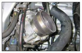
15. Install silicone hose number 084034 onto the throttle body and secure with the provided hose clamp.
