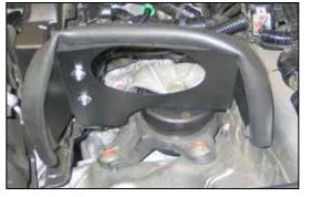
19. Install the heat shield and secure to the rubber mounted stud and bracket using the provided hardware.
