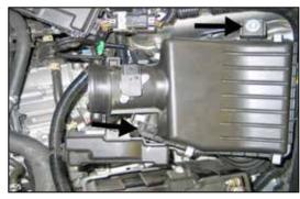
6. Loosen the two bolts securing the air box assembly to the inner fender and ECU bracket.
