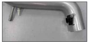
18. Install the mass air sensor into the K&N® intake tube and secure with the provided hardware.
