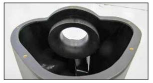
11. Install the K&N® filter adapter into the K&N® air box and secure with the provided hardware.
