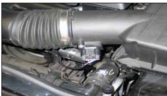
2. Disconnect the mass air sensor electrical connection.
