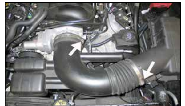
5. Loosen the hose clamps which secure the stock intake tube to the air box and throttle body.
