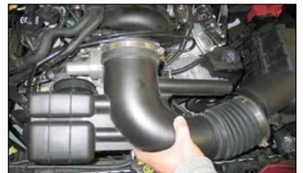
6. Remove the stock intake tube as shown.
