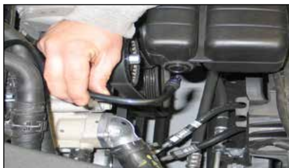
4. Disconnect the crank case vent tube from the intake resonator as shown.
