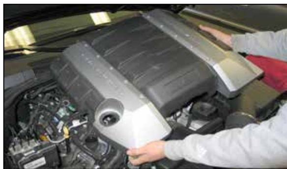
3. Remove the oil filler cap and then lift up and remove the engine cover. Reinstall the oil filler cap. NOTE: On 2014 and later vehicles, the manufacturer changed the crank case vent system. The crank case vent tube will need to be unhooked from the oil filler cap before the cap can be removed from the engine.
