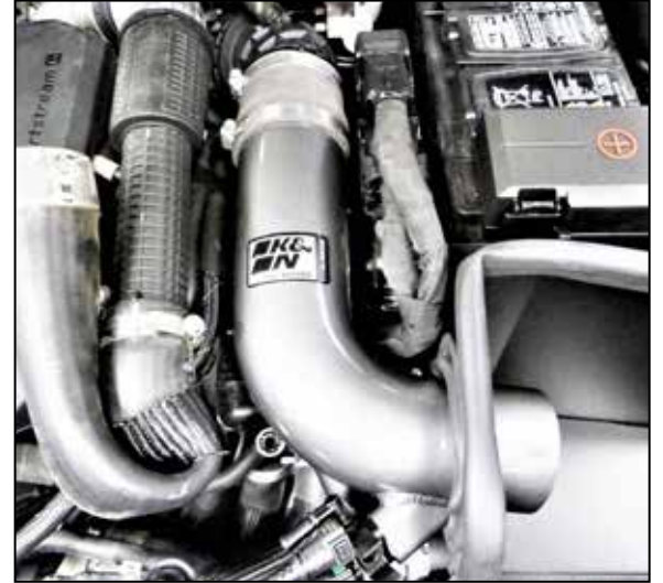
16. Install the K&N intake tube through the heat shield and into the coupler, align for best fit and then secure with the provided hose clamp.
