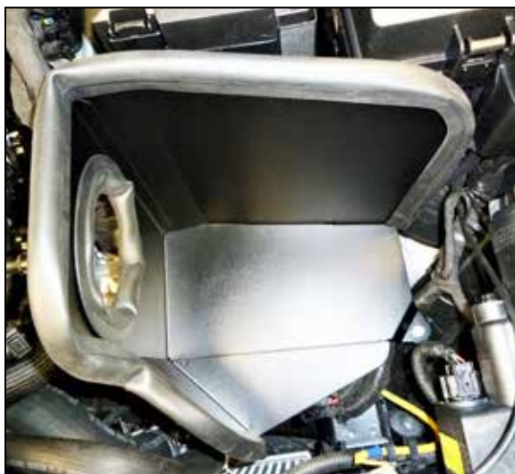
14. Install the heat shield assembly and secure it to the factory air filter housing mounting location using the provided hardware.
