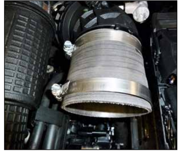
15. Install the provided coupler onto the turbo inlet pipe and secure with the provided hose clamp.
