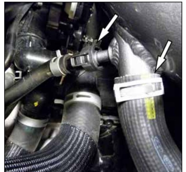
17. Connect the BOV hose and the vent line with the installed straight fitting onto the K&N intake tube as shown.
