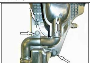
6. Remove the two push-pins that secure the fresh air duct to the air filter housing, release the locking tab and then rotate the duct counter clockwise to remove it from the air filter housing.
