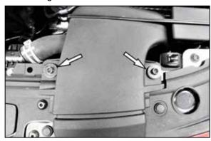
3. Remove the two bolts that secure the fresh air intake duct.
