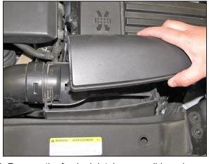
3. Remove the fresh air intake scoop lid as shown.
