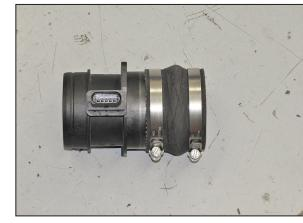
18. Install the provided coupler (087121) onto the mass air sensor and secure with provided hose clamp.
