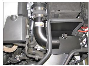
21. Install the K&N® intake tube into coupler on the mass air sensor and into the heat shield. Secure the intake tube to the bracket with the provided hardware and to the coupler with the provide hose clamp.
