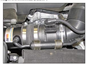
23. Reconnect the mass air sensor electrical connection and the vacuum line.
