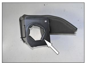
14. Install the 13" edge trim into the heat shield as shown.
