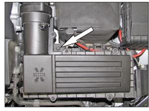
6. Loosen the bolt that secures the air filter housing to the vehicle.
