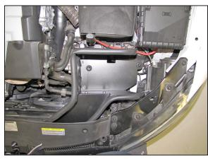
16. Set the heat shield into position on the air filter housing mounting studs and secure the bracket with the provided hardware.
