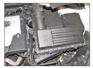
7. Release the spring clamp securing the intake tube to the mass air sensor, disconnect the warm air hose and then remove the air filter housing and mass air sensor from the vehicle.
