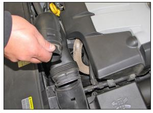
4. Disconnect the fresh air tube from the air filter housing and then remove the tube from the vehicle.
