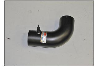
20. Install the provided vacuum fitting into the K&N® intake tube as shown.
