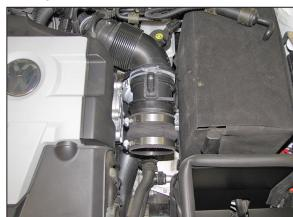
19. Install mass air sensor assembly onto the factory turbo inlet tube and secure with factory spring clamp.
