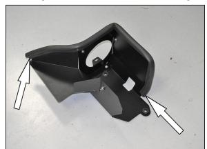
13. Install the 30" edge trim onto the heat shield as shown.
