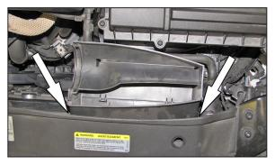
5. Remove the two bolts securing the fresh air intake scoop to the core support and then remove the scoop from the vehicle.
