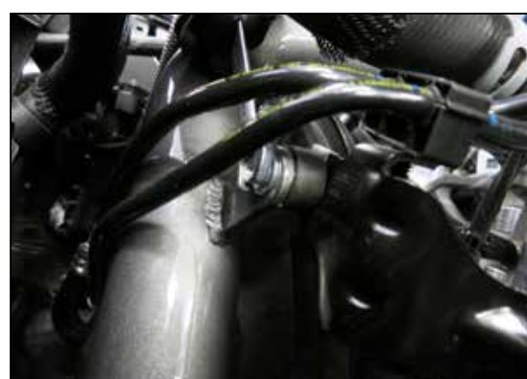
28. Insert the charge tube into the Coupler at the turbo outlet and the intercooler inlet hose, adjust the tube for best fit and then secure the hose clamps. Fully tighten the charge pipe mounting nut.
