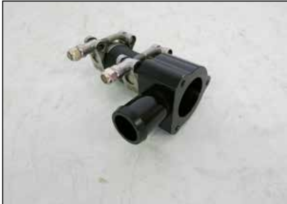
23. Install the provided BOV hose onto the K&N BOV manifold and secure with the provided hose clamp.
