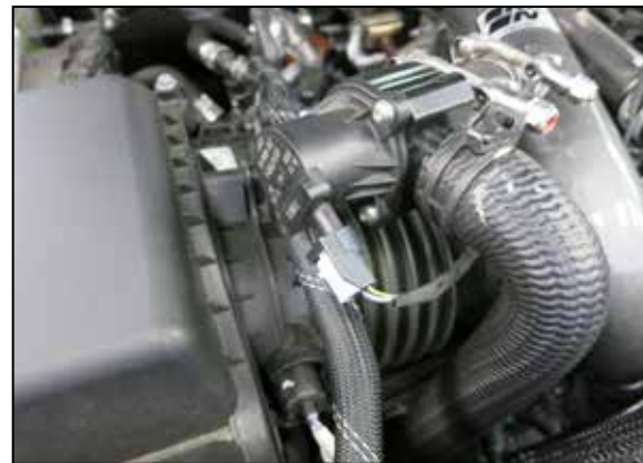
30. Reconnect the BOV valve electrical connection.
