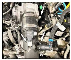
6. Disconnect the PCV quick connect fitting, disconnect the pressure sensor electrical connection, and then loosen the hose clamp securing the charge tube to the throttle body.
