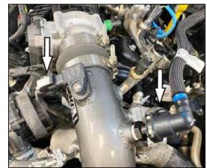
8. Remove the pressure sensor from the factory charge tube.
