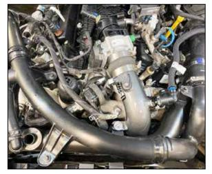
19. Reinstall the factory hot side charge tube and secure the factory clamps and hardware.
