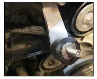
10. Install the provided rubber mounted stud onto the lower mounting bracket.
