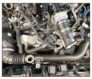
5. Remove the bolt that secures the intake tube to the engine, then loosen the two hose clamps and remove the intake tube from the vehicle.
