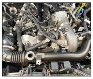
17. Reinstall the left side factory intake tube and secure the hose clamps.
