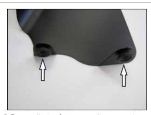
5. Remove the two factory mounting grommets from the factory air filter housing and install them into the K&N heat shield as shown.
