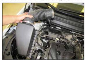
4. Loosen the hose clamp that secures the intake tube to the intake plenum. Disconnect the intake tube and then remove the complete intake system.
