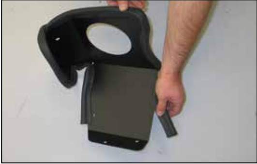
11. Install the provided edge trim onto the heat shield as shown. NOTE: Some trimming of the edge trim will be necessary.
