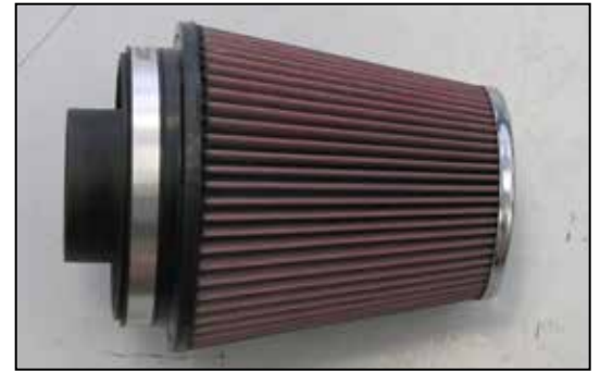
22. Install the filter adapter into the K&N® air filter and secure with the provided hose clamp.
