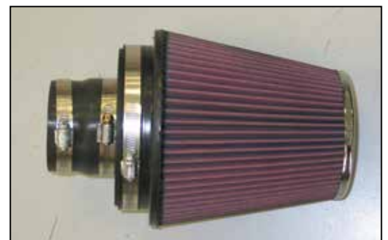
23. Install the silicone (08051) hose onto the filter adapter and secure with the provided hose clamp.
