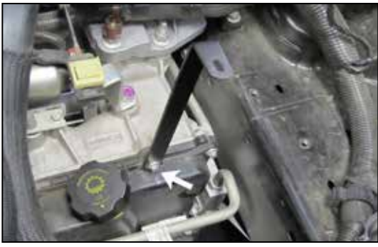
10. Install the intake tube mounting bracket (070095) onto the transmission pan and secure with the factory bolt removed in step #9.
