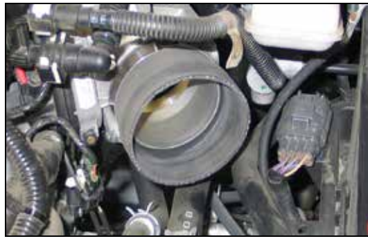
15. Install the silicone hose (084091) onto the throttle body and secure with the provided hose clamp.
