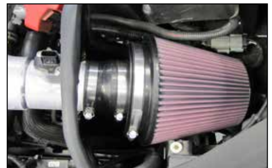
24. Install the filter assembly onto the intake tube and secure with the provided hose clamp. NOTE: Drycharger® air filter wrap; part # RF-1042DK is available to purchase separately. To learn more about Drycharger® filter wraps or look up color availability please visit http://www.knfilters.com ®.
