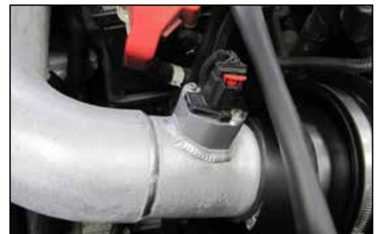
25. Using the provided mass air sensor extension harness, reconnect the mass air sensor electrical connection.
