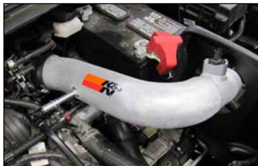
19. Install the K&N® intake tube into the silicone hose at the throttle body and align with the mounting bracket installed in step #10. Secure the intake tube with hose clamp and hardware provided.
