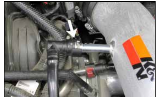
21. Connect the crankcase vent hose to the quick connect fitting on the K&N® intake tube as shown.
