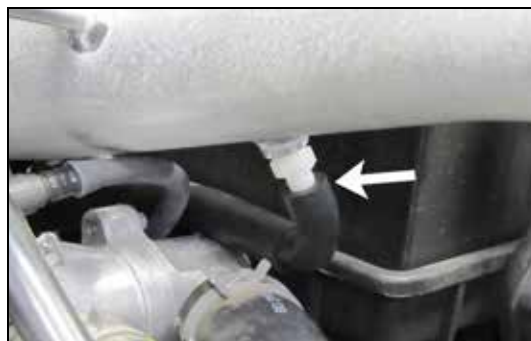
20. Connect the EVAP hose to the 1/4npt fitting as shown.
