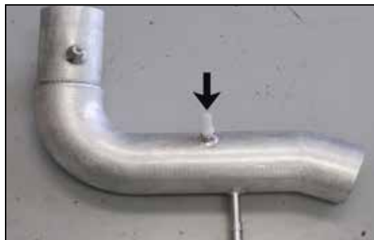
18. Install the provided 1/4npt fitting into the K&N® intake tube as shown. NOTE: Plastic NPT fittings are easy to cross thread. Install the vent fitting "hand" tight, then turn it two complete turns with a wrench.
