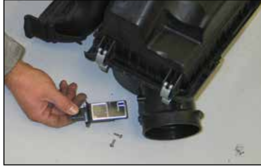
16. Remove the two screws securing the mass air sensor to the airbox and then remove the mass air sensor from the airbox.
