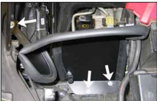
14. Install the heat shield into position on the inner fender and secure with the factory airbox mounting bracket bolts removed in step #8. Secure the heat shield mounting bracket to the airbox mounting bracket location on the core support using the factory bolt removed in step #5. NOTE: On 2007 and 2008 model year vehicles, secure the wiring harness to the "L" bracket installed during step #12.
