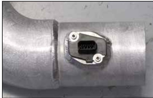
17. Install the mass air sensor into the K&N® intake tube and secure with the provided screws.
