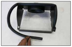
10. Install the bulb edge trim to the top of the heat shield as shown. Some trimming of the edge trim will be necessary.
