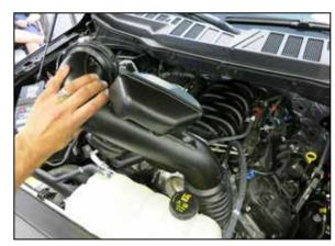
5. Remove the intake tube and upper air filter housing from the vehicle.
