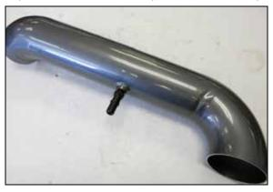
16. Install the provided quick connect fitting into the intake tube as shown.
