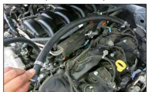
12. Install the CCV assembly onto the engine. NOTE: the 90deg fitting will be attached to the engine.
