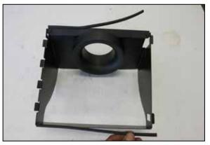
9. Cut the provided small edge trim into two sections and install onto the heat shield as shown using the provided super glue to lock it into position.
