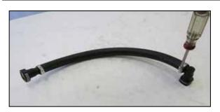
7. Assemble the provided CCV hose assembly using the hose, fittings, and clamps.
