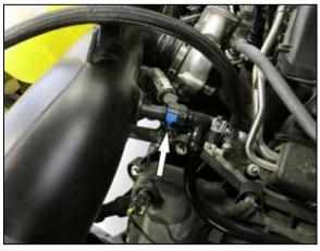
4. Disconnect the CCV from the factory intake tube.
