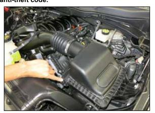
2. Release the two locking tabs that secure the upper air filter housing.
