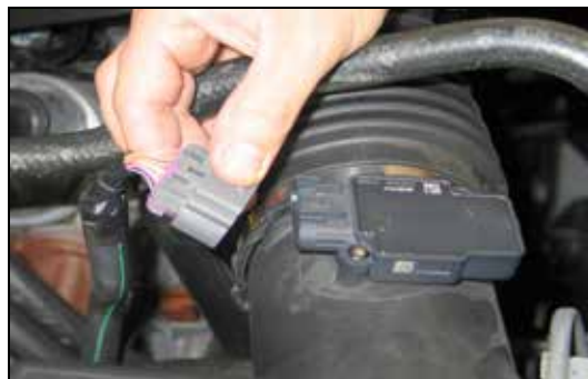
2. Disconnect the mass air electrical connection.
