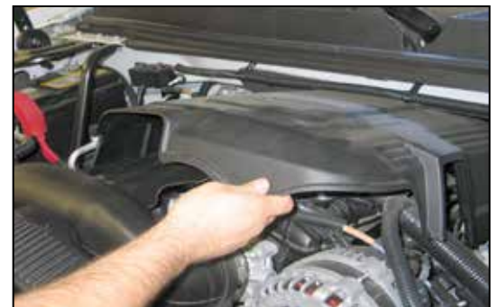
3. Lift up on the engine cover and remove as shown.
