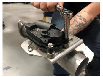
6. (FOR AFM VALVE DELETE ONLY) Align and secure both of the factory AFM valve actuators to the CORSA AFM delete assemblies using a 10mm socket and a ¼" ratchet. Torque to 89 IN-LBS.
