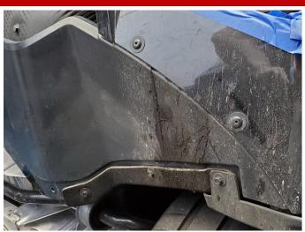
The rearward most rear under tray is secured by two push clips (1 per side), four T15 TORX screws (2 per side), and six 7mm bolts (3 per side). Remove the push clips first using a removal tool or flathead screwdriver, followed by the T15 TORX screws, and then the bolts using a 7mm socket and 1/4" ratchet. This will free the rearward under tray from the vehicle. Set aside the rearward under tray and fasteners in a protected location.
