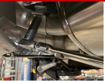
**32.** Rotate the CORSA inner tip elbow pipe until it is centered in the rear valence, then tighten the exhaust clamp at the elbow pipe inlet using a 15mm socket and 3/8" ratchet.
