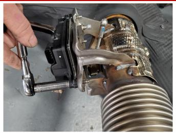
29. Remove the six bolts (3 per side) that secure both of the factory AFM valve actuators using a 10mm socket and a ¼" ratchet. Set aside the AFM valve actuators in a protected location. The AFM valve actuators will be reused during the installation of the CORSA exhaust system.
