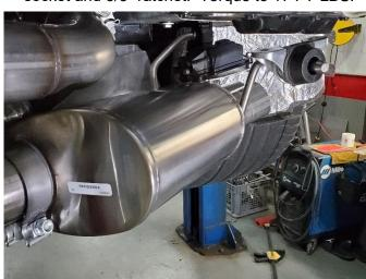
24. Repeat Install Steps 19-23 for the passenger side of the vehicle. (CORSA passenger muffler shown)
