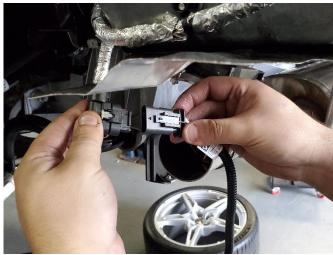
**26.** (FOR NPP VALVE ONLY) Locate both NPP valve wiring extensions from the hardware kit. Connect both wiring extensions to the chassis side of the NPP valve wiring connectors. Push in the grey locking tabs on the wiring connectors to secure the connections.
