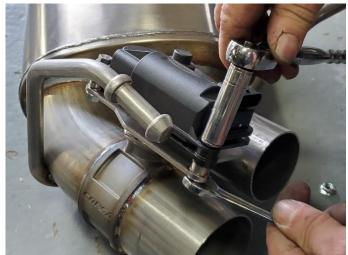
17. (FOR NPP VALVE ONLY) Locate the two CORSA NPP compatible muffler (or muffler delete) assemblies, and the two stock NPP valve actuators set aside in Removal Step 26, along with the remaining six supplied M6 bolts and M6 nuts from the hardware kit. Align and secure both of the factory NPP valve actuators to the CORSA NPP valve assemblies using a 10mm socket, a ½" ratchet, and a 10mm wrench. Torque to 89 IN-LBS.
