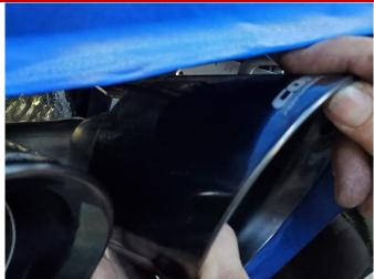
**35.** Locate one of the CORSA inner tip assemblies, and a 2.5" clamp from the hardware kit. Position the clamp on the tip inlet so the clamp bolt is on top of the tip and the clamp nut is facing inwards. Insert the inlet of the inner tip assembly onto the elbow pipe with approximately 1.5" of overlap.
