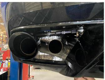
34. Adjust the rotation of the CORSA outer tip assembly until the CORSA logo is centered on the top of the tip, then tighten the exhaust clamp at the tip inlet using a 15mm socket and 3/8" ratchet.
