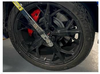
7. Remove the ten lug nuts and the two rear wheels from both sides of the vehicle using a 22mm socket and ½" ratchet or ½" drive breaker bar. This will allow access to the factory inner fender liners. Set aside the rear wheels and lug nuts in a protected Location.
