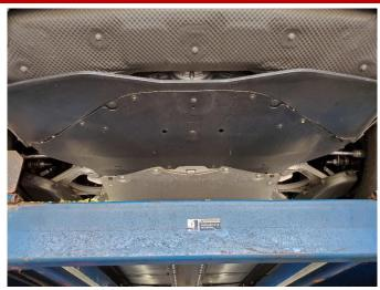
5. The forward most rear under tray is secured by one push clip and ten 7mm bolts. Remove the push clip first using a removal tool or flat head screwdriver. Next, remove the bolts using a 7mm socket and 1/4" ratchet to free the forward under tray from the vehicle. Set aside the forward under tray and fasteners in a protected location.
