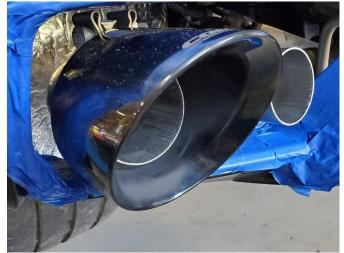
**33.** Locate one of the CORSA outer tip assemblies, and a 3" clamp from the hardware kit. Position the clamp on the tip inlet so the clamp bolt is on top of the tip and the clamp nut is facing inwards. Insert the inlet of the outer tip assembly onto the elbow pipe with approximately 1.5" of overlap.
