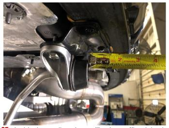
25. At this time, adjust the muffler (or muffler delete), X-pipe, and head pipe positions until there is approximately ½" between the outer face of the rear grommets and the forward edge of the head on the rear hangers on both driver and passenger sides of the vehicle as shown. It is critical for proper fitment to get the system adjusted a square as possible on the vehicle.
