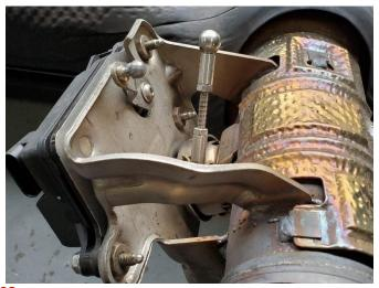
**28.** Remove both of the AFM valve actuator linkages from the AFM valve actuators and the stock AFM valve assemblies.
