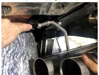
**21.** Insert the driver front muffler (or muffler delete) hanger into the front exhaust grommet as shown.
