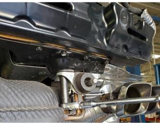
**18.** Support the factory exhaust with a jack stand. Remove the four bolts that secure both of the rear exhaust grommets to the chassis using a 13mm socket and 3/8" ratchet. Set aside the fasteners in a protected location.
