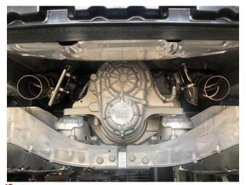
10. Pivot and rotate the driver side head pipe assembly at the flange connection until the AFM valve actuator position mirrors the passenger side on both height and rotation as shown.
