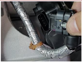
12. Reconnect the wiring connectors to both of the AFM valve actuators. Push in the grey locking tabs on the wiring connectors to secure the connections.
