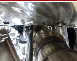
8. Secure the passenger side cat back mounting flange to the factory catalyst using a 13mm socket, a 3/8" ratchet, and a 24" long extension. Torque to 17 FT-LBS.
