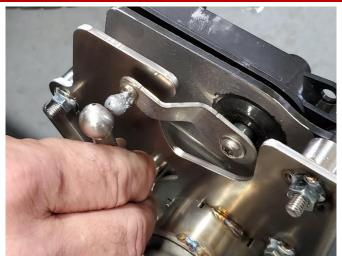
(FOR AFM VALVE ONLY) Connect both of the AFM valve actuator linkages to the factory AFM valve actuators. Secure the connections with the remaining locking pins.
