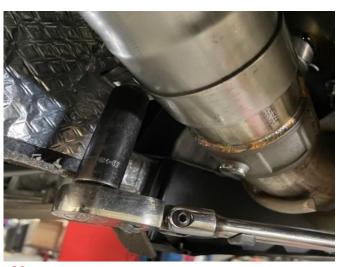
**30.** Rotate the CORSA outer tip elbow pipe until it is centered in the rear valence, then tighten the exhaust clamp at the elbow pipe inlet using a 15mm socket and 3/8" ratchet.
