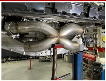
15. Adjust the rotation and overlap of the X-pipe assembly onto both of the head pipes until the Xpipe outlets are even both vertically and front to back in the vehicle. The X-pipe should be centered on the midline of the vehicle behind the rear differential.
