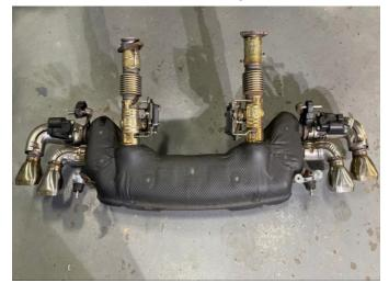
**23.** CAREFULLY slide the factory exhaust down and rearward to free it from the vehicle.
