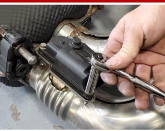
**26.** (FOR NPP VALVE ONLY) Remove the six bolts (3 per side) that secure both of the factory NPP valve actuators using a 10mm socket and a ¼" ratchet. Set aside the NPP actuators in a protected location. The NPP valve actuators will be reused during the installation of the CORSA exhaust system.
