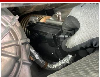
22. Disconnect the wiring connectors to both of the AFM valve actuators; these are located on the inside of the head pipes between the muffler and the factory catalysts. Note that the grey locking tab on the wiring connectors must be slid outwards before disconnecting the wires from the actuators.
