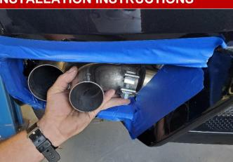
**31.** Locate one of the CORSA inner tip elbow pipes, and a 2.5" clamp from the hardware kit. Position the clamp on the elbow pipe inlet so the clamp bolt is facing towards the bend and the clamp nut is facing downwards. Insert the inlet of the elbow pipe onto the non-valved outlet of the driver side muffler with approximately 1.375" of overlap.
