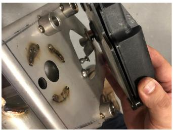
5. (FOR AFM VALVE DELETE ONLY) Locate the two CORSA AFM delete head pipe assemblies, and the two stock AFM valve actuators set aside in Removal Step 29, along with the six supplied M6 bolts from the hardware kit. Insert the actuator arm through the window in the CORSA AFM delete assembly as shown.
