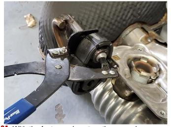
24. With the factory exhaust on the ground, remove the front grommets from the exhaust hangers using a grommet puller or similar device. Once again, the use of a soap and water solution will aid in the removal of the hangers from the factory grommets. Note the orientation of the grommets for the installation of the CORSA exhaust system.
