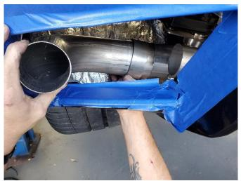
29. (ALL VERSIONS) Locate one of the CORSA outer tip elbow pipes, and a 3" clamp from the hardware kit. Position the clamp on the elbow pipe inlet so the clamp bolt is facing away from the bend and the clamp nut is facing downwards. Insert the inlet of the elbow pipe onto the valved outlet of the driver side muffler with approximately 1.75" of overlap.
