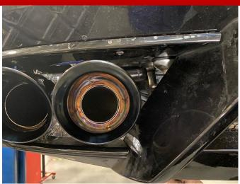
**36.** Adjust the rotation of the CORSA inner tip assembly until the CORSA logo is centered on the top of the tip, then tighten the exhaust clamp at the tip inlet using a 15mm socket and 3/8" ratchet.
